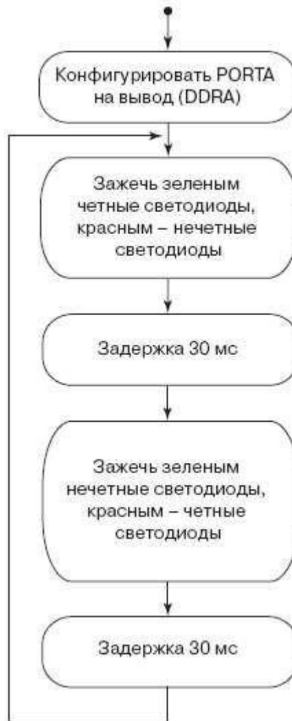
Fig.4. Block diagram of the LED control algorithm
