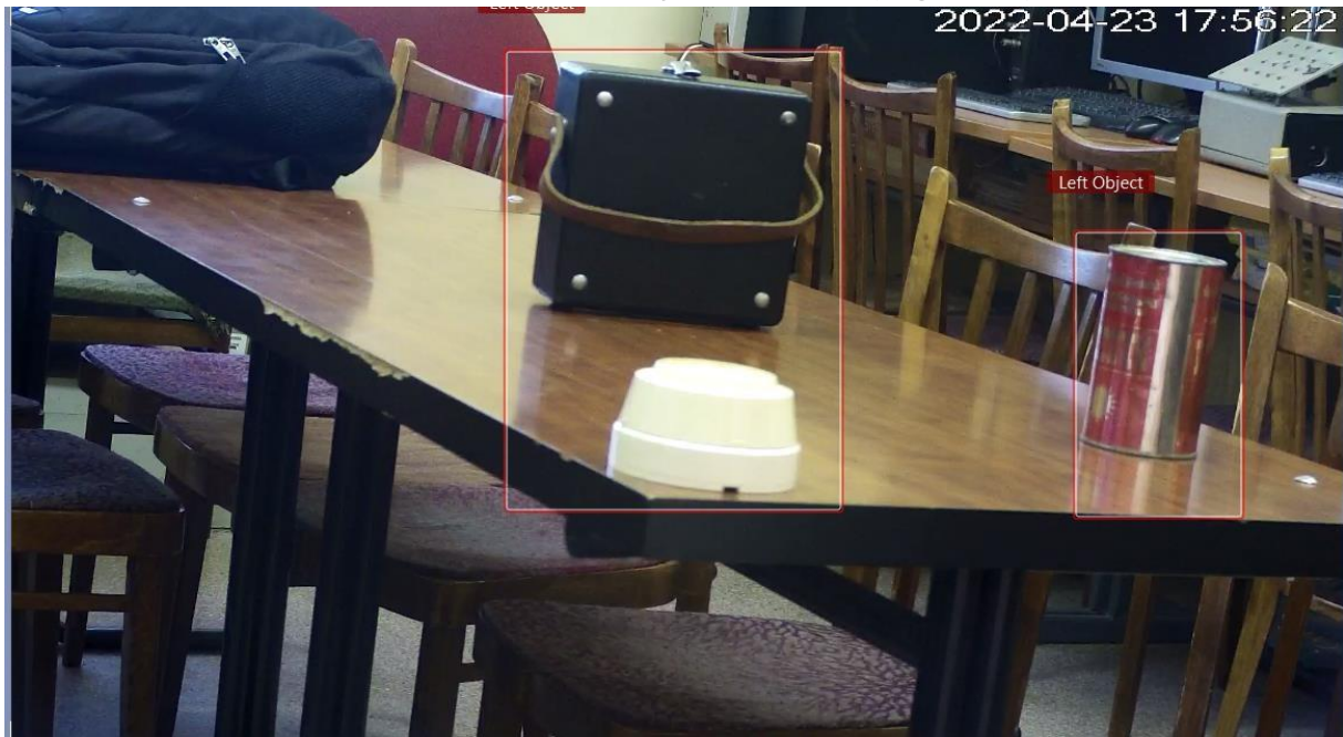
Figure 3.24 – Selecting two objects as one abandoned object If you leave the objects 15 seconds after there was no one abandoned object, then we get 4 correctly detected objects, 1 undetected (video camera) and 1 false detection (Fig. 3.25).
