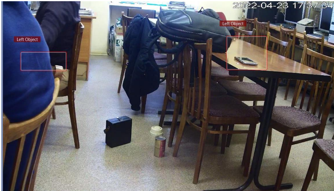
Figure 3.22 – Identification of several abandoned objects An increase in the sensitivity of the algorithm leads to an increase in false Triggers: one item out of four was correctly detected (Fig. 3.23).
