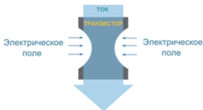
Figure 11. Principle of operation of a field-effect transistor
