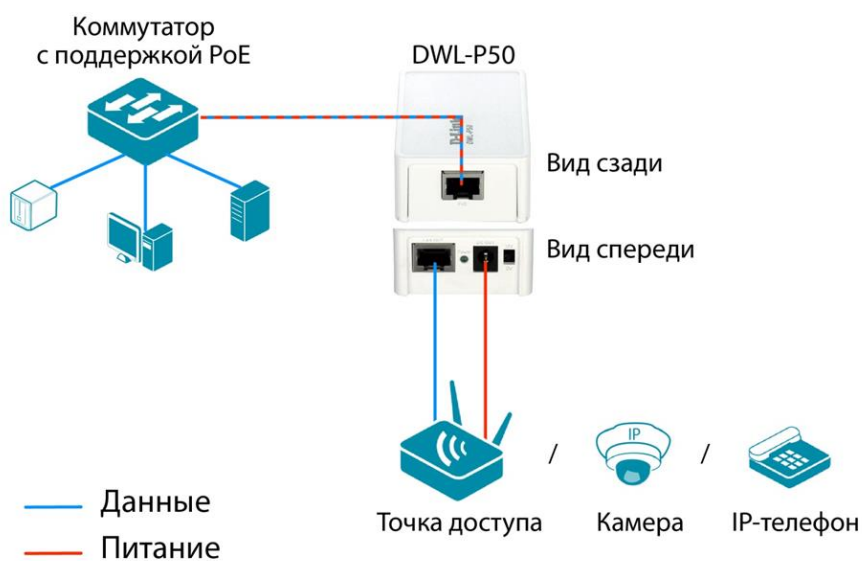
Figure 4. Simplifying the installation of network devices
