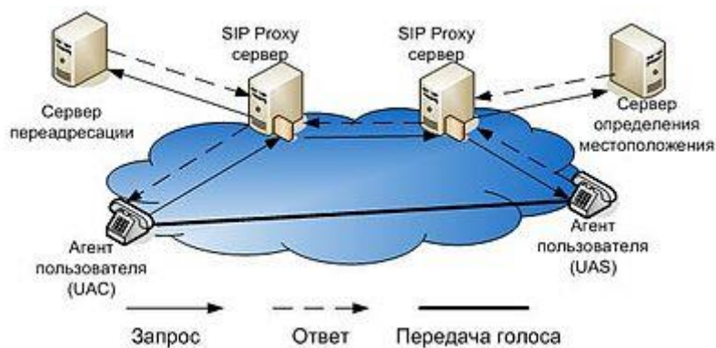
Figure 2. Structural diagram of a connection using the SIP protocol
