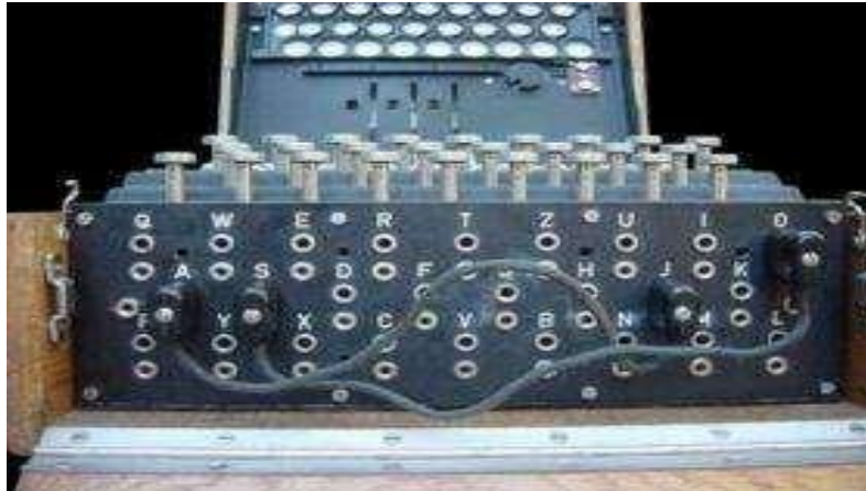
Fig. 3.8. The patch panel at the front of the machine. Up to 13 connections could be used. In the photo, two pairs of letters are switched (“S”-“O” and “J”-“A”)
