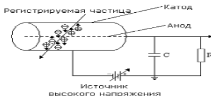
Figure 2.4 – Schematic Diagram of GC Design (Registered particle; Cathode; Anode; High-voltage source)
