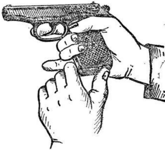
Fig. 3. Removing the magazine from the grip frame
