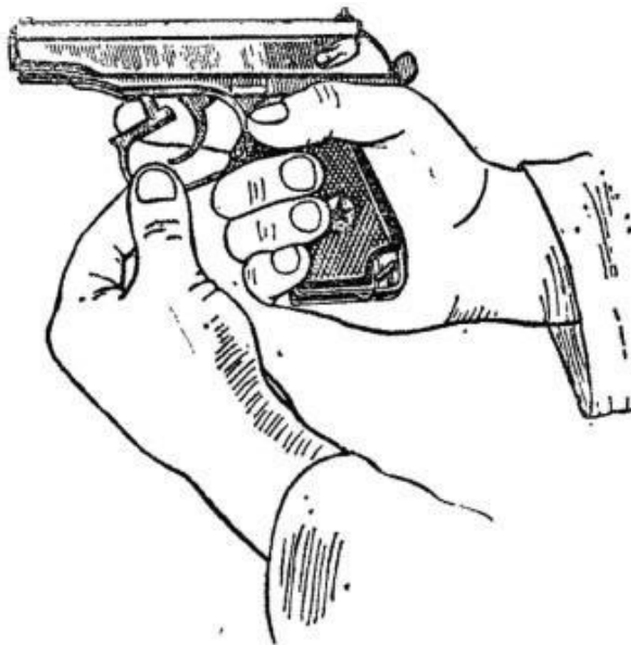
Fig. 4. Pulling down the trigger guard
