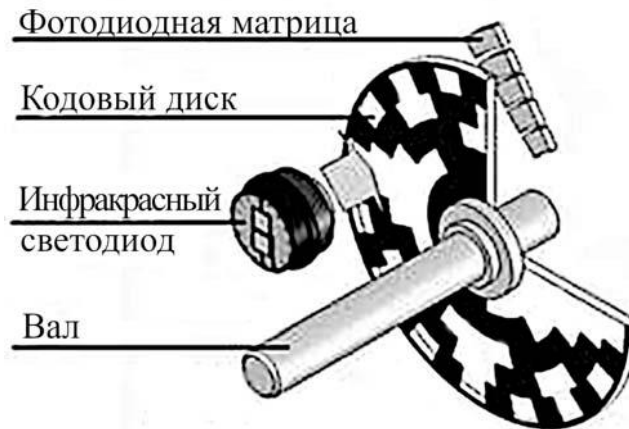
Figure 2.3 – Single-turn encoder design
