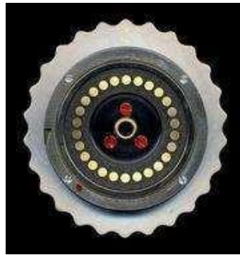
Fig. 3.3. Left side of the Enigma rotor, planar electrical contacts are visible
