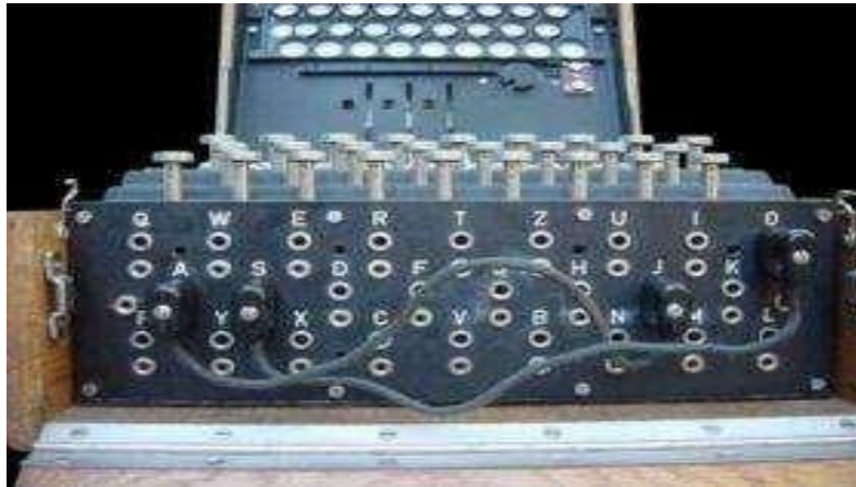
Fig. 3.8. Patch panel at the front of the machine. Up to 13 connections could be used. In the photo, two pairs of letters are switched ("S"-"O" and "J"-"A")
