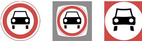
Fig. 2.10 — On the left — the original image, in the center — barrel distortion, on the right — pillow-shaped distortion.
