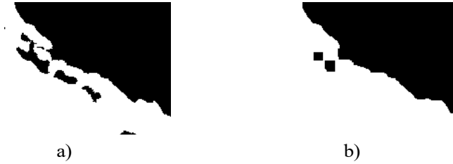
Fig. 4.9 — a) The result of the execution of the bwareaopen() function; b) the result of the execution of the imclose() function.
