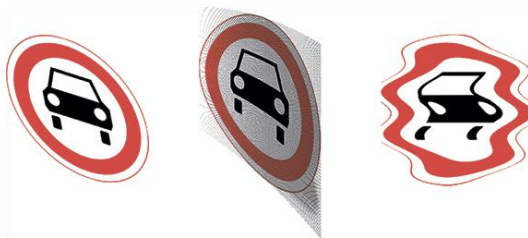
Fig. 2.8 — Polynomial distortion on the left, projective distortion in the center, and sinusoidal distortion on the right.
