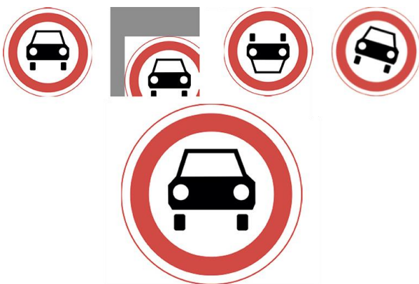
Fig. 2.2 — Conformal transformations, top row from left to right: original image, shift, reflection, rotation; bottom row: homogeneous scaling.
